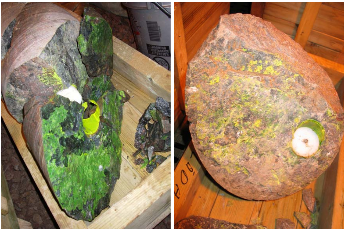
Figure 3-2. Feature A in KXTT3 (to the left) and in KXTT4 (to the right). The green material is uranine tagged epoxy.
