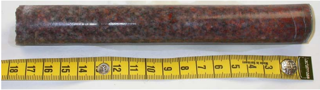
Sample core drilled from the fracture surface on the core stub
